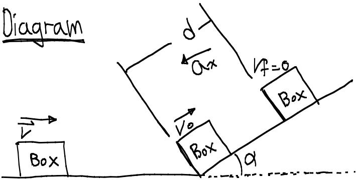
A box was initially pushed and push force was removed. The box starts up the inclined plane with velocity of  $V_0$  and travels distance  $d$  to stop its motion
